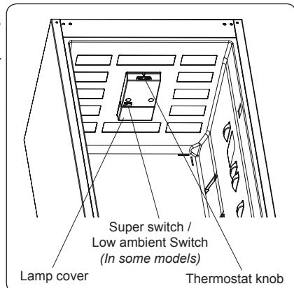
**Super freezing:** This switch shall be used as superfreeze switch. For maximum freezing capacity, please turn on this switch before 24 hours placing fresh food. After placing fresh food in the freezer, 24 hours ON position is generally sufficient. In order to save energy, please turn off this switch after 24 hours from placing fresh food.
